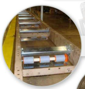
Re-build: Install new conveyor components onto existing framework
